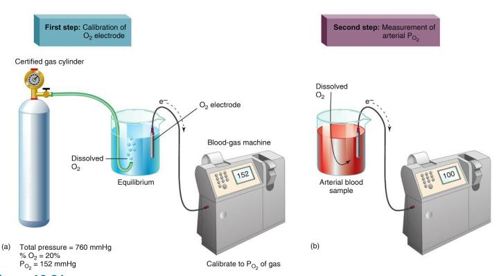
**Figure 16.21** Blood gas measurements using the  $P_{o_2}$  electrode. (a) The electrical current generated by the oxygen electrode is calibrated so that the needle of the blood gas machine points to the  $P_{o_2}$  of the gas with which the fluid is in equilibrium. (b) Once standardized in this way, the electrode can be inserted into a fluid such as blood, and the  $P_{o_2}$  of this solution can be measured.
