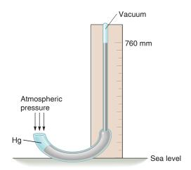
**Figure 16.18** The measurement of atmospheric pressure. Atmospheric pressure at sea level can push a column of mercury to a height of 760 millimeters. This is also described as 760 torr, or one atmospheric pressure.
