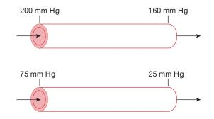
5. All four tubes below have the same driving pressure. Which tube has the greatest flow? Which has the least flow? Defend your choices.
