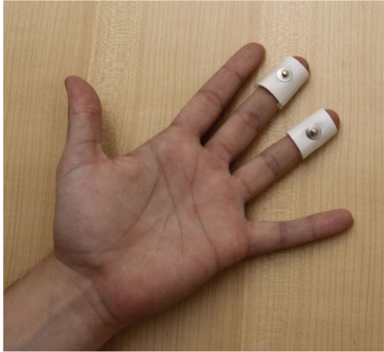
Fig. 1 Electrodermal activity electrode placement on the third phalanx of the middle and ring fingers of the participant's nondominant hand
