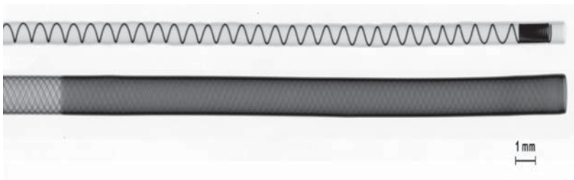
Figure 6.10 X-ray image, showing internal support structure of catheters from Figure 6.9.
