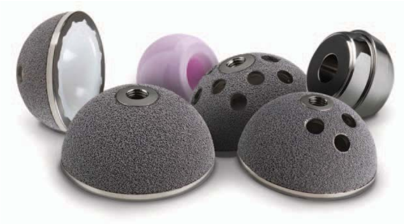
Figure 12.8 A modular trabecular metal acetabular cup system (Zimmer, Inc., Warsaw, IN). The same acetabular porous ingrowth cup, with or without holes for screws, may be used with a variety of polyethylene, ceramic, or highly polished metal liners (cups). This allows the liner, in some material combinations, to be replaced in subsequent revision surgeries with a new, unworn component, without needing to remove a potentially well fixed, porous ingrowth shell. This also allows a surgeon to switch to a larger ball diameter, by replacing the femoral ball and the acetabular liner, without having to compromise a potentially well-fixed acetabular cup with bony ingrowth.
