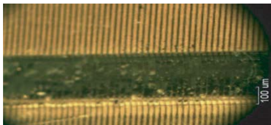
Figure 14.22 Piezoelectric slab diced into a 128-element linear array.
