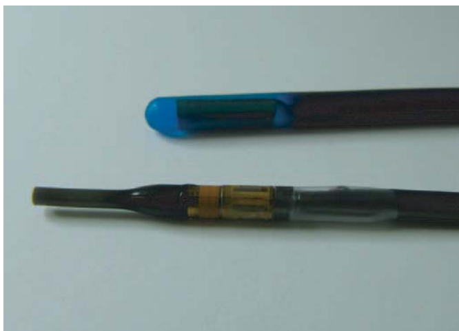
Figure 14.29 Linear phased array ICE catheter, with elements arranged in the long dimension of the catheter (top), and radial phased array IVUS catheter, with elements arranged around the circumference of the catheter (bottom).
