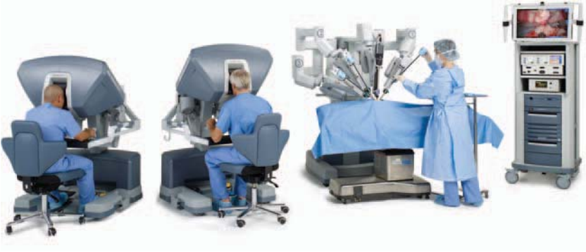
Figure 5.10 The da Vinci Si by Intuitive Surgical Inc. (a) Surgeon-side two surgical console and (b) Patient-side subsystem. Source: © 2012 Intuitive Surgical, Inc.
