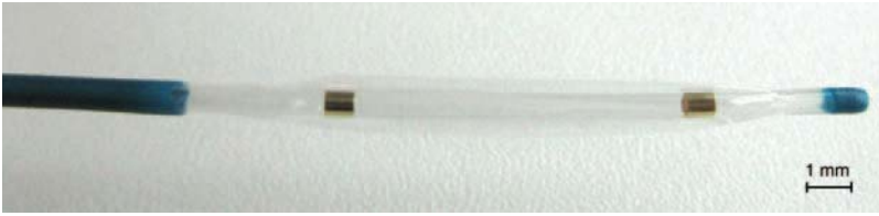
Figure 6.7 A traumatic tip and X-ray marker of a balloon catheter.
