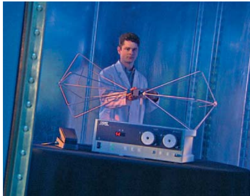
Figure 2.8 Assessment of new electronic device designs often entails electromagnetic radiation testing to ensure that its operation will not interfere with other devices.
