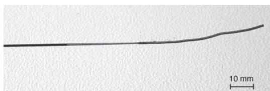
Figure 6.19 Guide wire with 0.018 in. diameter and a springlike tip.
