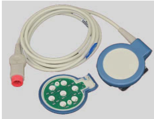
Figure 14.33 External fetal heart monitor (top) and disassembled external fetal heart monitor, with seven piezoelectric elements incorporated onto a circuit board (bottom). Source: Courtesy of Tenacore Holdings, Inc.
