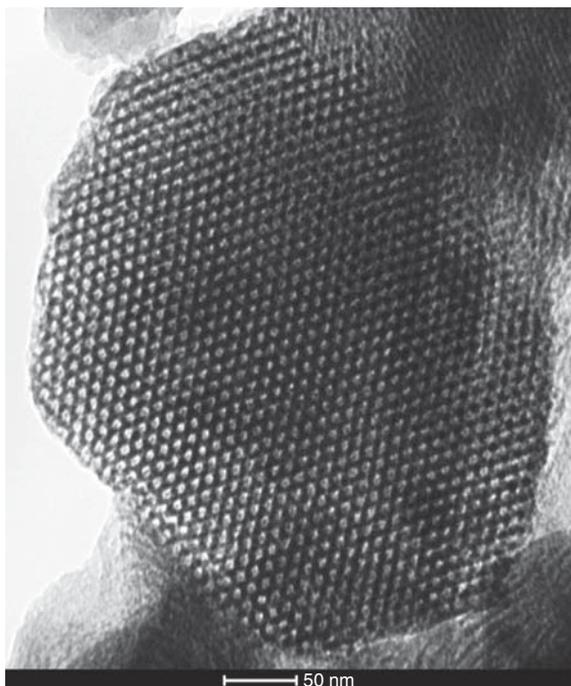
**Figure 8.6** TEM micrographs of iron oxide nanoparticles on mesoporous aluminosilicates synthesized via a dry-milling protocol. Reproduced with permission from Ref. [25].
