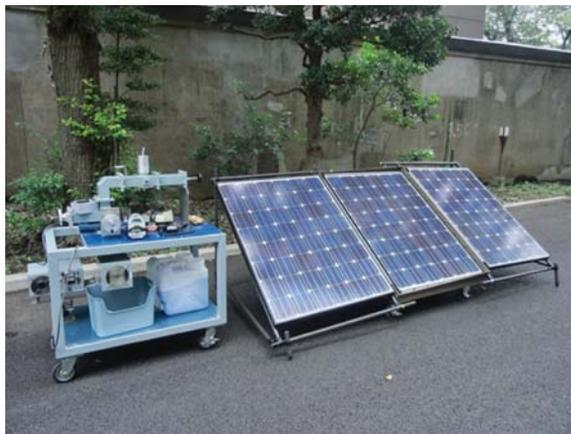
**Figure 19.12** Water sterilization equipment used to sterilize natural water (accumulated rain water) samples using the solar cells located on the right-hand side of the photograph and the  $\text{TiO}_2$ -coated MDELs (150 pieces) [32] Copyright 2014 by S. Horikoshi and N. Serpone.
