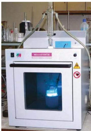
**Figure 8.4** MW/UV combined technology with EDL lamps. Reproduced with permission from Ref. [22].
